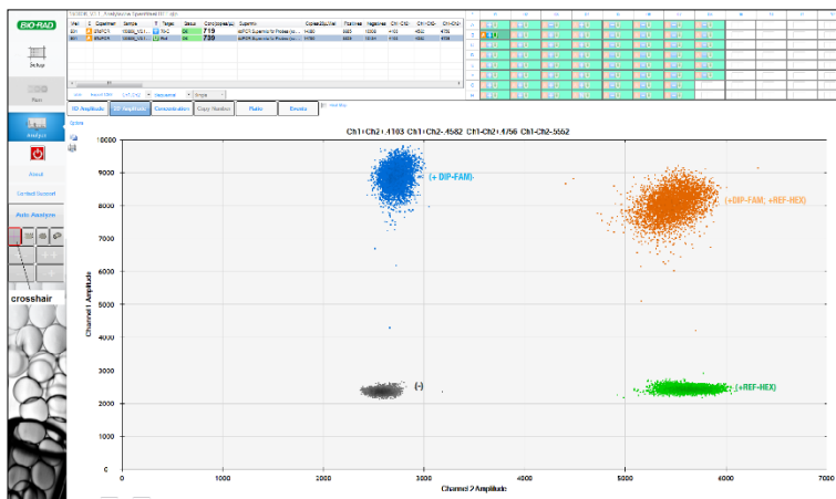
Figure 4 2D amplitude view (scatter plot) of the droplet fluorescence
